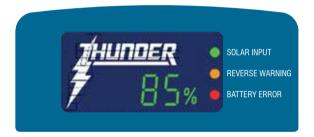
**NOTE:** The percentage display shows the stage at what the DC-DC battery charger is in, not the percentage of the battery charge, at 80% the battery is fully charged.
