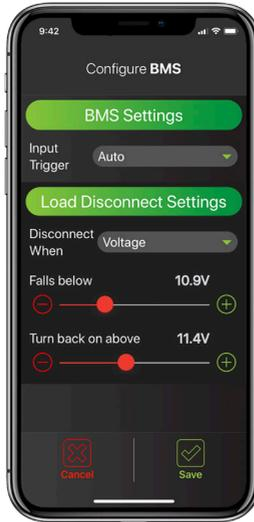
The Configure BMS (Charger) page allows you to setup the Input Trigger and Disconnect When settings for a Manager30 should one be connected.
