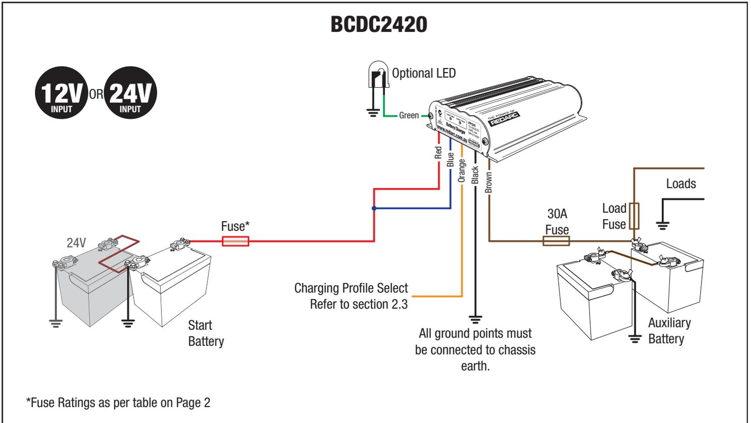
Figure 2.8a - BCDC2420 Standard setup for a 12V or 24V Start Battery
