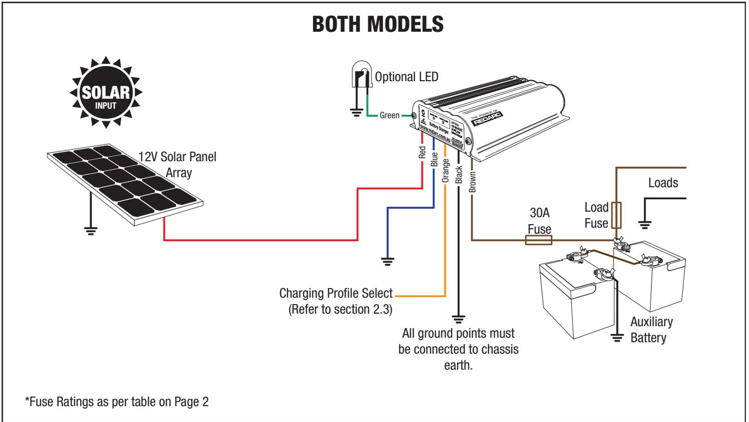
Figure 2.8c - Both Models Standard setup for a 12V Solar array
