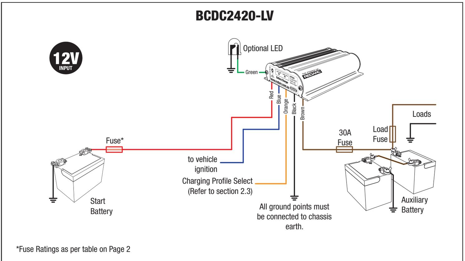
Figure 2.8b - BCDC2420-LV Standard setup for a 12V Start Battery
