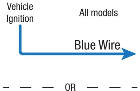
For standard (non 'LV') models, the BLUE wire may be permanently connected to the Input Source Positive supply and the charger will only charge when the alternator is running. This is not suitable for the BCDC2420-LV.
