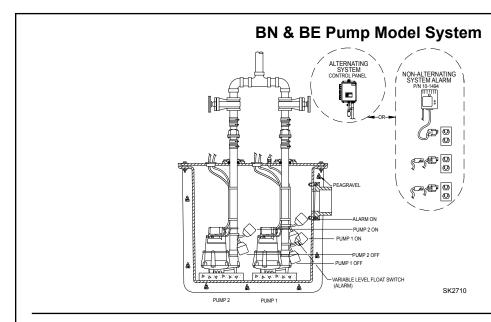
Note: Lead and lag pump can be altered by switching pump power cord to opposite switch outlet.
