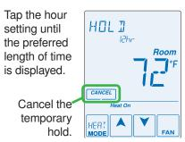
'HOLD' is displayed while the thermostat is operating at the temporary hold temperature. Energy savings can be achieved by lowering the heating temperature and increasing the cooling temperature when the building is unoccupied or during the night.
