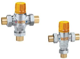
In solar systems, the temperature in the storage tank can vary considerably, depending on the solar radiation, and can reach very high temperatures over long periods. In summer, and if there is little water usage, the hot water at the storage tank outlet can actually reach temperatures around 200° F. At these temperatures, the hot water cannot be used directly because of the danger of scalding. Function
