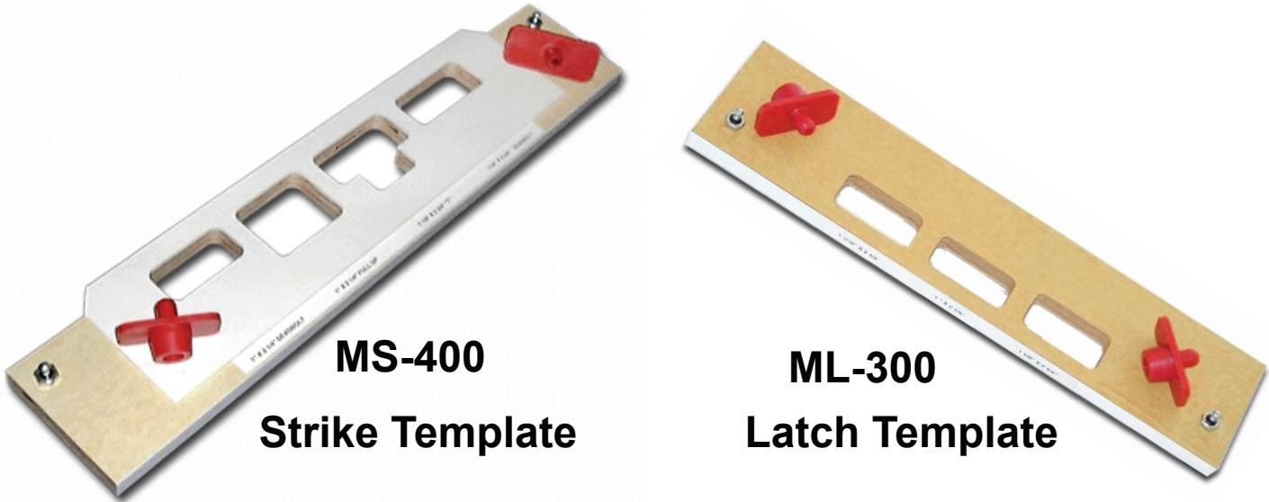
Instructions for using both of these templates is virtually the same. The red plastic center locators and the red plastic stops on the underside of the template are used in the same way. The strike template is used on the door jamb and the latch template is used on the edge of the door. Follow the instructions below using a 1/2" hinge mortising bit and a 5/8" OD template guide on your router to create the proper mortises for your jamb and door.
