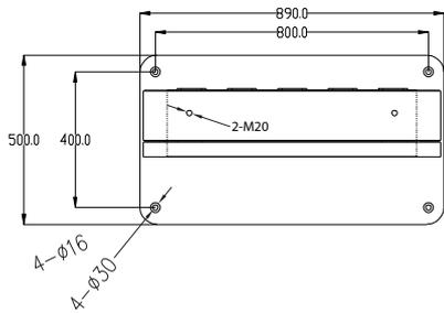
Note: The  $\phi 30$  holes are for access, we recommend using M10 anchor bolts that will fit into the  $\phi 16$  holes.
