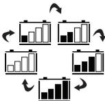
**Boost/CC charging** – All bars are continuously filling up in a cycle.
