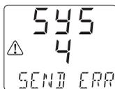
**SYS 4** – In the event there is a transmission issue during the configuration procedure and the Charging Device cannot be programmed a corruption error is detected and the Remote Display will indicate **SEND ERR**. A transmission error is often caused by a fault with the Data Cable or the connections. See note 2.
