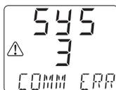
**SYS 3** – If there is a data exchange issue between the Charging Device and the Remote Display, a damaged Data Cable for example, a communications error is detected and the Remote Display will indicate **COMM ERR**. See note 1 & 2.
