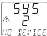
**SYS 2** – If only one Charging Device is connected and the **[AB]** button is pressed (to toggle between Charging Devices) a connectivity error is detected and the Remote Display will indicate **NO DEVICE**. See note 1.
