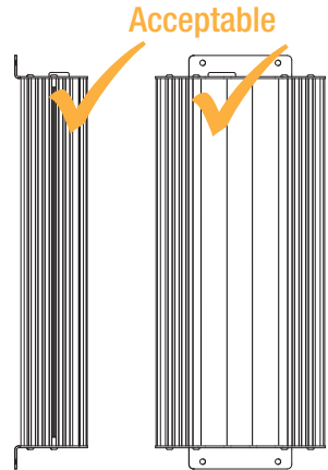
Figure 2.2.1.2 - Vertical mounting is acceptable
