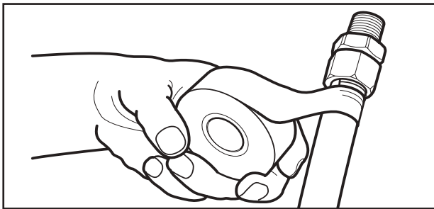
Figure: 4-17 Wrapping with self bonding silicone tape - begin on jacket.
