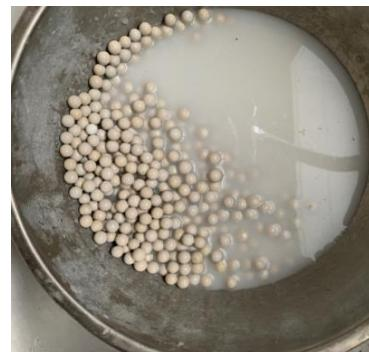
Figure 6: Neutralization media that has been rinsed with clean water
