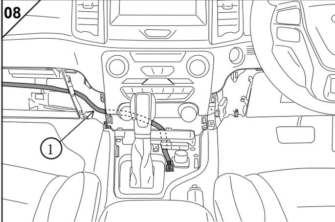
Route the Remote Head cable (1) along existing wiring (forward of glovebox hinge) to the area to the Right Hand Side of the Gear shift.
