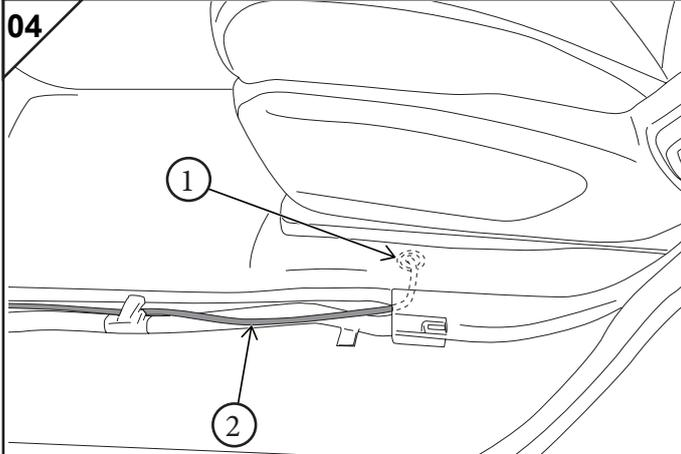
Locate the 40mm grommet (1) under the Passenger Front seat (under carpet) and discard.
