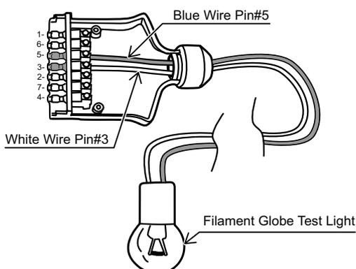
Test the installation using a test load (recommended 21W globe or equivalent) between terminal 5 and 3 on the trailer socket.
