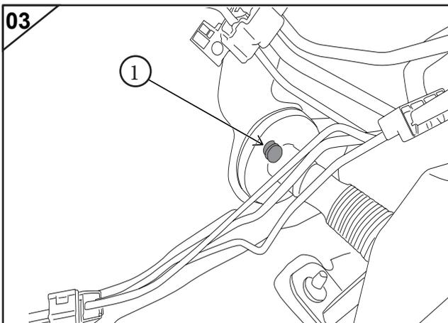
In the Engine Compartment in front of the passenger, pierce the end of the main grommet nipple (1), and feed the terminal end of the fused BLACK wire through to the interior.
