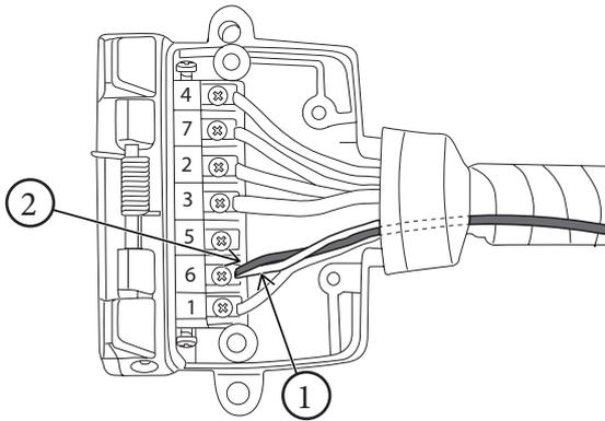
Open the trailer socket (7-pin shown as example); remove any cable clamp and peel back boot (if fitted).
