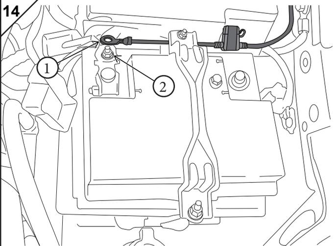
Secure BLACK fused wire (1) to existing wiring, connecting the eyelet to the Positive terminal (2).
