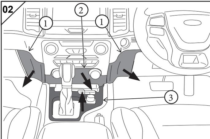
Remove both centre console lower Side Trims (1) and then Lower Centre Console (2) (fixings exposed).
