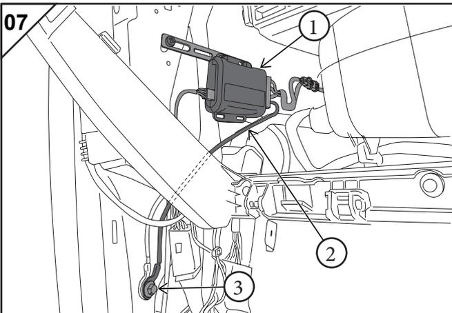
Secure the Main Unit (1) to the left hand side of the glovebox:
