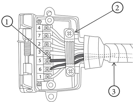
If any BLUE is fitted to terminal 5 position, remove and insulate, pulling back to main harness.
