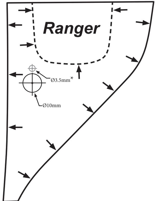
\* The 3.5mm hole is not required for the V3 head
