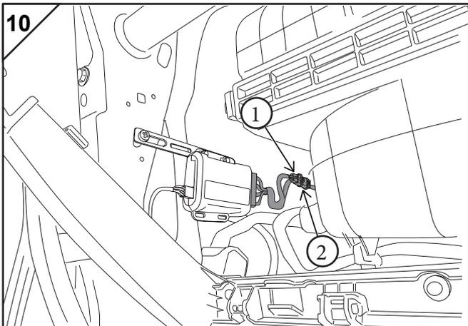
Connect small 'Signal Conditioning Module' (1) supplied in kit, to the small 2-way connector near the 4-way Power MOLEX, ensuring you hear the 'click' of engagement, and secure to wiring with two cable ties (2).
