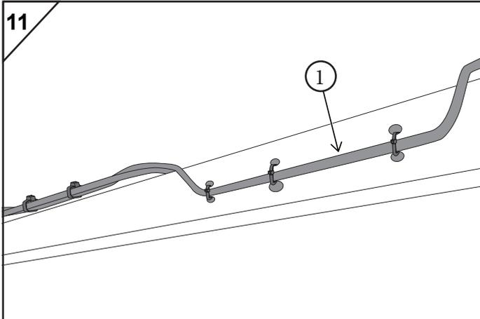
Under the vehicle, route the TWIN CORE BLUE/RED cable (1) along the chassis rail rearwards, securing to existing vehicle wiring where possible. If no wiring near, feed cable ties through chassis holes and secure wiring to side face, as indicated left.
