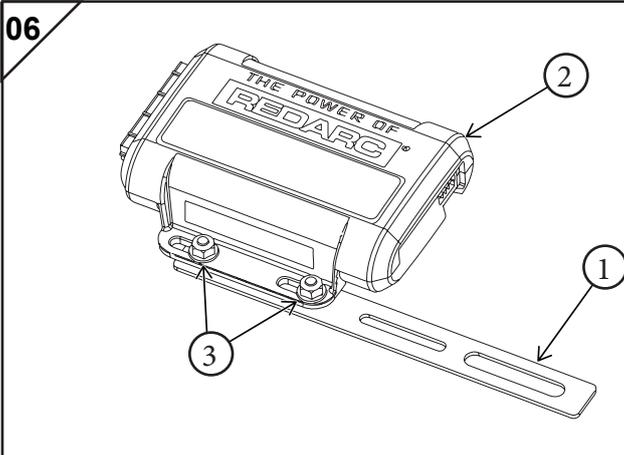
Fit the bracket strap (1) to one side of the Main Unit (2) using the fixings provided, as shown left (3).
