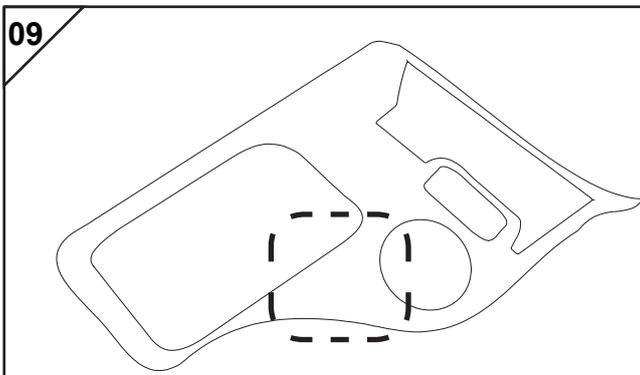
Using the drilling template provided, drill the mounting hole(s) and then fit the Remote Head to the gear surround trim from behind, securing with the nut provided.
