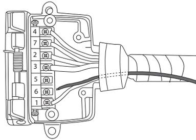
At the Trailer Socket, remove the existing RED wire at terminal #6 and pull outside the wiring harness.
