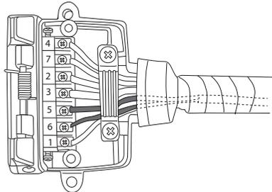
Feed both the exposed RED and BLUE wires (at the end of the main cable) into the Trailer Socket.
