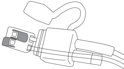
Feed this removed RED wire into the supplied joiner in the rubber boot at the end of the twin-core cable.
