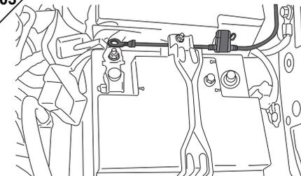
Run the BLACK fused Positive supply wire from the Vehicle Start Battery positive terminal through the cabin entry point to the Main Unit location.
