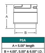
Use as a connector between appliance exhaust collar and the positive twist lock of "L" Vent pipe.
