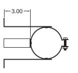
Provides exterior, vertical/lateral support for chimney. Maxiumum height of chimney which can be supported is 30 feet.
