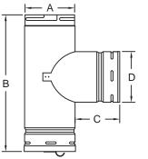
SIZE В С D Α 4" 4.50" 10.13" 3.00" 4.50" 3.00" 5.50" 5" 5.50" 11.13" 6" 6.50" 12.13" 3.00" 6.50" Use tee to transition from horizontal to vertical inside or to an exterior chimney that is mounted to a tee support.
