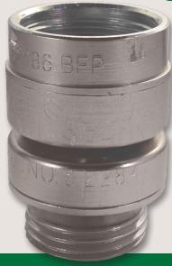
Arrowhead Brass Self-Draining Vacuum Breakers are made of Lead-Free brass and provide protection against back-flow caused by back-pressure siphonage while also allowing water inside the valve to drain upon shut off, providing protection from freezing. Arrowhead Brass Self-Draining Hose Vacuum Breakers are available in brass and polished chrome finishes and includes a breakaway set screw for permanent installations.
