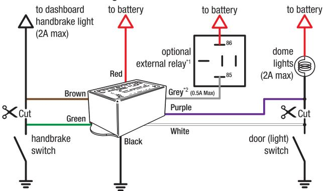
Please note that a combination of the two wiring diagrams may be used to suit vehicles with either positive door and negative handbrake switches, or negative door and positive handbrake switches.
