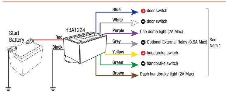
The Handbrake Negative input (Green wire) has specific operating voltage requirements. Care should be taken if other circuits, electronic controls or power circuits are connected to this input which may cause voltages other than battery positive or negative. The following specification applies:
