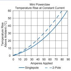
NOTE: Powerclaw charts are based on #8 AWG equivalent copper foil on board side, mated to #6 AWG conductor on wire side.
