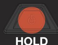
HOLDING the Power Button will put the screen into Standby mode. Pushing any button will wake the screen up again. When the system is set to 'Storage Mode' only the Power Button will wake the display up.
