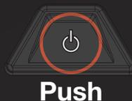
Pushing the Power Button ONCE will open a Power Button instruction dialogue and allow switching between Storage and Touring modes.
